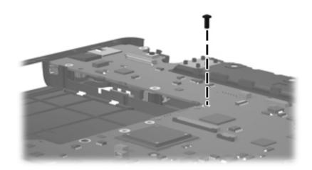
Where used: 1 screw that secures the system board to the base enclosure
